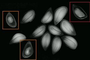
AI defect classification — orange: embryo defect · red: severe defect
